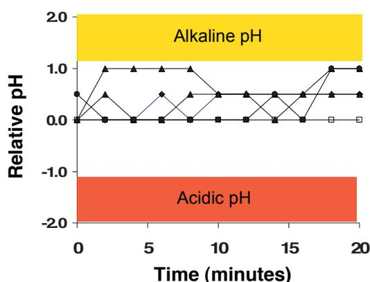
**Figure 2:** Timecourse of pH excursions relative to the starting pH for six electrodes. Electrode polarity was negative; total dose was 80 mA\*minutes
