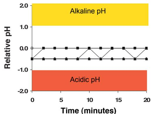
**Figure 1:** Timecourse of pH excursions relative to the starting pH for six electrodes. Electrode polarity was positive, total dose was 80 mA\*minutes.
